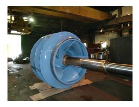
**Project Description:** The purpose of this project is to refurbish one main sewage pump rotating assembly at the RAPS. The work includes complete disassembly, inspection of the impeller for re-use, and replacement of the shaft and all other parts. Epoxy coating of the impeller is an added technical feature. The project will provide for refurbishment of this assembly and return it to a condition where it can provide another lifecycle of utilization.
