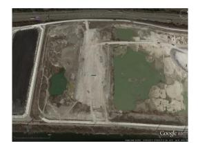
**Project Description:** The expanded Stage 2 portion of the McCook Reservoir replaces the originally planned Stage 3 and expands the reservoir to include former sludge drying lagoons 21 and 22 at the Lawndale Avenue Solids Management Area. This project will remove the overburden on lagoons 21 and 22 to allow for the underlying rock to be mined.
