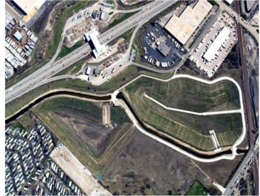
**Project Description:** Restore eroded slopes, spillways, outflow channels, gabions, damaged concrete, and joints at the Touhy Avenue Reservoir in accordance with 2011 to 2015 inspection reports and permit requirements.
