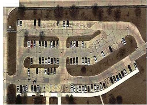
**Project Description:** Demolition of the existing concrete parking lot, driveways, storm sewers, and other associated appurtenances. Installation of a new permeable paver parking lot, concrete driveways and walkways, underdrain system, bio-retention basin, landscaping, and energy-efficient parking lot lighting.
