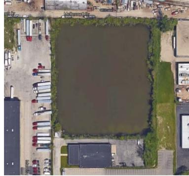
**Project Description:** Construct two new storm sewers along McDermott Drive and Morris Avenue, expand the existing detention basin, and construct a stormwater pumping facility at the southwest corner of the existing detention basin to adequately convey a 100-year storm event. This is a cost sharing agreement with the Village of Berkeley.
