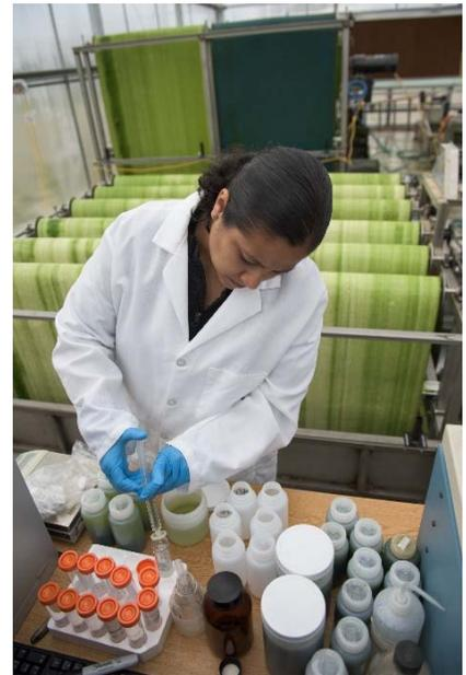
Lab Tech I Maricela Sabido demonstrates the algae process for nutrient removal.
