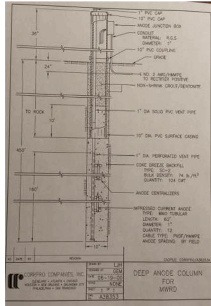
**Project Description** Drill four, 10-inch diameter, holes by approximately 400 feet. Furnish, deliver, and install 14 mixed metal oxide sacrificial anodes in the four holes. Fill the remainder of the holes with coke breeze and bentonite. Install new junction boxes. Connect new wires to the existing rectifier system. Install reference cells for the new deep anode ground bed cathodic protection system in the east and west TARP pumping stations. Replace conduit and cables as needed.
