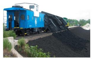
Biosolids are delivered by train from the Stickney Water Reclamation Plant to the Lawndale Avenue Solids Management Area, where they are mixed with wood chips to produce high quality compost.
