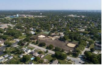
In Western Springs' Springdale Park, the MWRD is helping fund construction on a supplemental storm sewer system and storage basin that is expected to mitigate flooding in the area through the MWRD's Stormwater Partnership Program. The project benefits approximately 20 homes and two local roads by providing adequate drainage to depressional areas of the neighborhood and detention for excess stormwater runoff.
