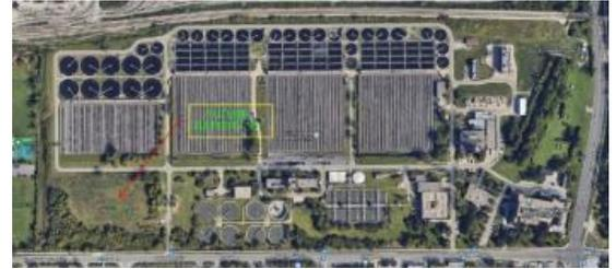
**Project Description** This project will remove the overburden soil pile at the southwest corner of the O'Brien WRP that needs to be removed to prepare the site for construction of a new battery. The soil pile covers approximately 10 acres, and its volume is approximately 120,000 cubic yards. A portion of the soil includes some contamination that will require hauling to a contaminated soil disposal/remediation facility.
