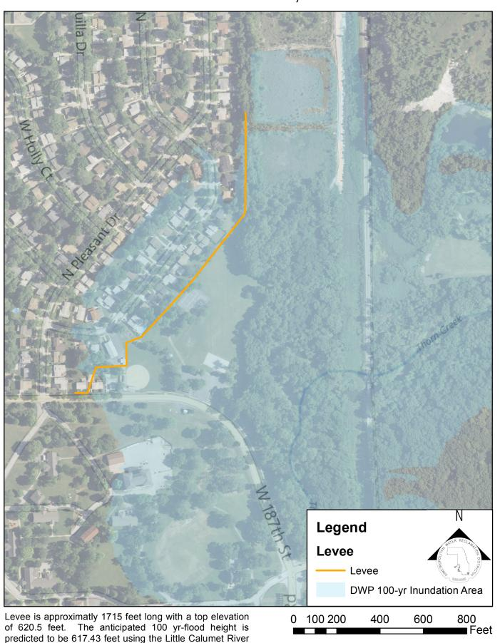
Detailed Watershed Plan models. The levee is expected to eliminate flood damages up to the 100-yr event for 31
