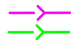
PROPOSED TRUNK LINE STORM SEWER (TO BE INSTALLED BY IDOT - 60" DIA.) PROPOSED LOCAL STORM SEWER EXTENSIONS (BETWEEN 15" AND 24" DIA.)
