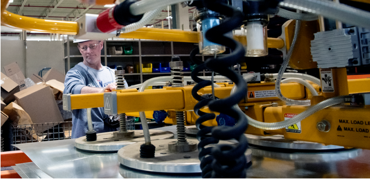
Storekeeper Michael Chester pulls steel plate with a vacuum lifter.
